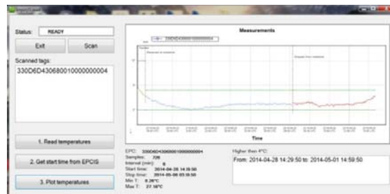
Fig. 8 Temperatures read from RFID data logger in the box
